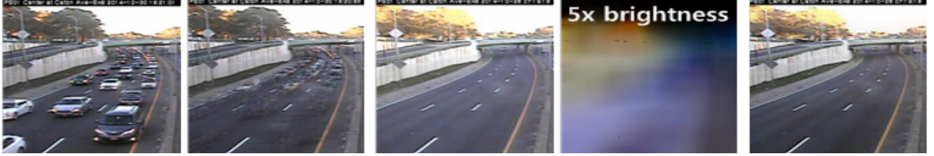
Fig. 2: From left to right: a) frame in heavy traffic; b) noisy GMM-generated background; c) reference picture of empty road; d) map of brightness adjustment; e) resulting clean background.
