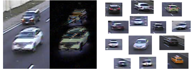
Fig. 4: left: original frame fragment with and without subtracted background (car ‘ghost’); right: examples of car patches for training cascade detectors
