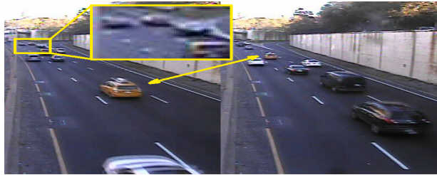
Fig. 1: A pair of sequential frames; one car correspondence is shown for clarity, smallest seen cars are 10 pixels.
