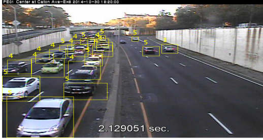
Fig. 5: Example of combining the two cascade detectors and the background subtraction based detector
